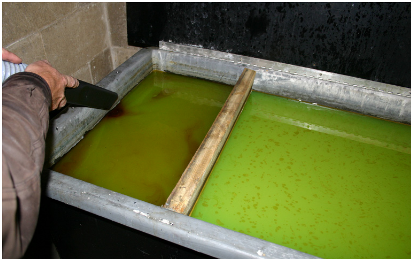
Machine Coolant & Drawing Compound TRAMP OIL floating on water squeezed to one end of the tank and removed with vacuum suction to maintain solution longevity, cleaning efficiency and consistent quality control.
