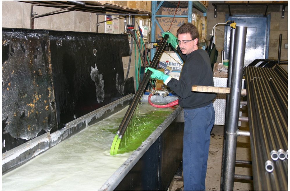
Machine Coolant & Drawing Compound contamination removed externally by immersion and internally by flushing in alkaline cleaner with multi-metal corrosion inhibition.
