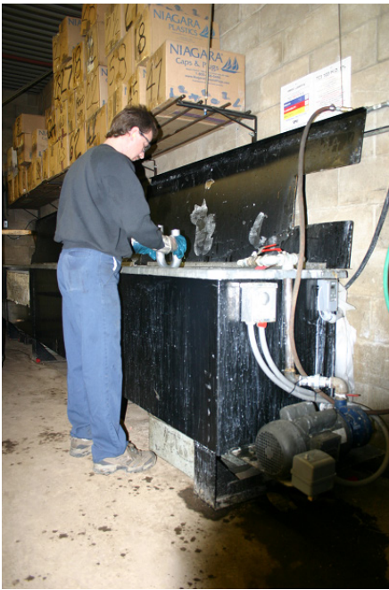
Machine Coolant & Drawing Compound contamination removed externally by immersion and internally by flushing in alkaline cleaner with multi-metal corrosion inhibition.
