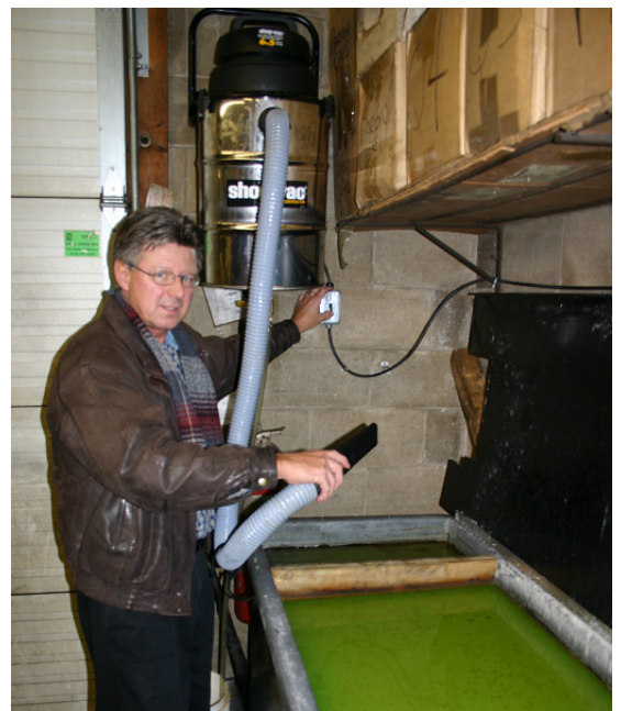
Machine Coolant & Drawing Compound TRAMP OIL floating on water squeezed to one end of the tank and removed with vacuum suction to maintain solution longevity, cleaning efficiency and consistent quality control.
