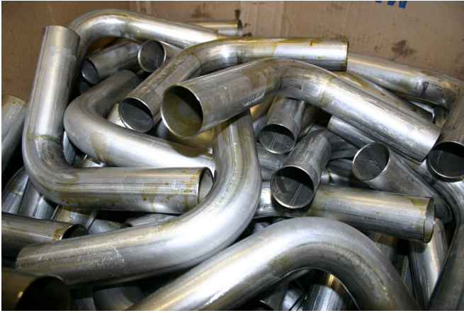
Machine coolant & drawing compound contamination
