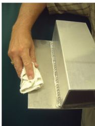
2) Wipe seam of aluminum to be welded
